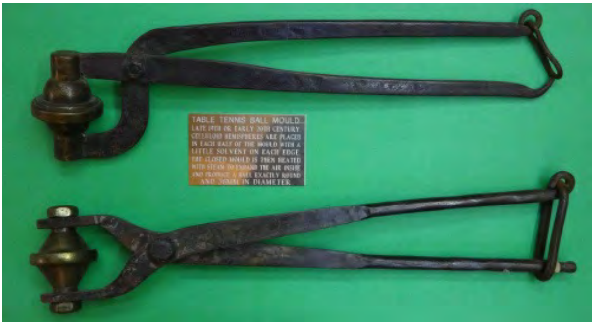
Old celluloid ball-making tools. The technique was described: “Celluloid hemispheres are placed in each half of the mould with a little solvent on each edge. The closed mould is then heated with steam to expand the air inside and produce a ball exactly round and 38mm diameter.”
